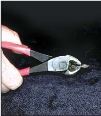
Fig 1.32a | Metal cutting pliers can cut only aluminum bands. They will only slightly dent the stainless steel band shown here.
