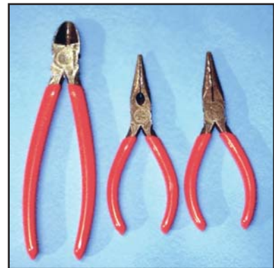
Fig 1.32f | Side cutters and needle-nose pliers are examples of tools used to cut bands and hold metal for bending or cutting.
