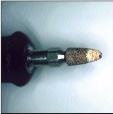
Fig 1.26a | Beak and nail trimming. The stone on this electric hand-held rotary tool® has been “loaded” with plastic or paint by grinding such a surface in such a manner as to “load” the stone, creating a smooth surface. This smooth surface generates heat for cautery if a beak or nail starts to bleed during trimming.
