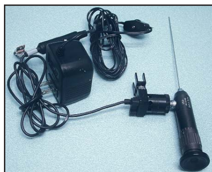
Fig 1.16f | Alternatively, an electrical plug can run the unit instead of battery power. The total unit price is several thousand dollars less than a traditional light source and flexible fiberoptic cable.
