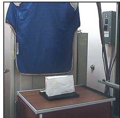
Fig 1.17c | Bird in bag on the cassette being exposed.
