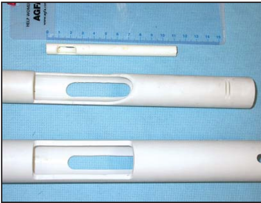
Fig 1.37 | Sections of plastic pipe used to make a speculum with a hole through which a gavage device can be passed.
