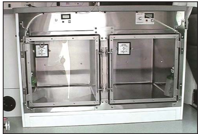
Fig 1.12c | Intensive care cages with heat, humidity, oxygen and nebulizer capabilities in the mobile clinic.
