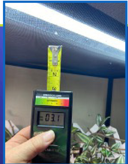
Figure 6 The ideal UVI of 3.0 measured by the Solarmeter 6.5R is achieved at 3"/7.6 cm. from the cage top and then decreases rapidly to unacceptable levels. An animal sitting more than 3" away from the top would receive inadequate levels of UVB even with a brand-new bulb.
